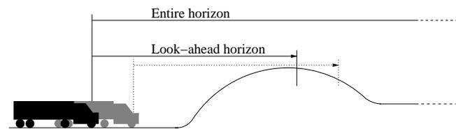
A tailored dynamic programming algorithm is currently used for the optimization. On the standard portable computer used in the experiments, tenths of a second are needed to calculate a solution for a typical horizon of 30 steps of 50 m that gives 1.5 km look ahead.
